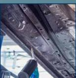
After 15-20 minutes – but no longer than 30 minutes –, the underbody must be treated with a DINITROL underbody protection product without exceeding or falling short of a layer thickness of 300 μm – 500 μm.
