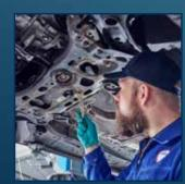
Next, the vehicle must be inspected. Flaking rust and all deposits must be removed.
