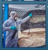
After treating the underbody, the cavities in the rear lid and bonnet must be sealed. Please ensure that the engine and boot are completely covered.
