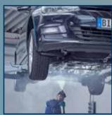
We recommend using a degreasing agent and high-pressure cleaner to thoroughly clean the vehicle in order to remove all soiling and flaking corrosion.
