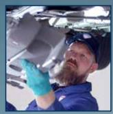
In the first step, all plastic parts must be removed from the underbody, wheel arch liners, and door panels.
