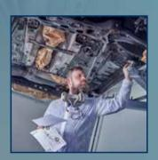
After the vehicle has been properly cleaned and prepared for treatment, carefully study the DINITROL spray diagram for the vehicle to be treated. This is the only way to avoid damage to the electrical system, airbags, and other sensitive parts.
