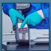
To maintain a continuous flow without stopping the gun, set the dosage regulator to zero (= 0).
