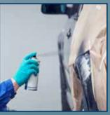
Spray **DINITROL 6900** onto the sanded surface in order to detect unevenness more easily. Now sand again until the **DINITROL 6900** is no longer visible.
