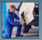
The area around the edges must be protected carefully with tape and paper. The damaged spot needs to be cleaned throroughly with a cleaner, such as **DINITROL 7660**, a quick-drying cleaning agent and silicone remover
