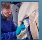
Next, apply the putty evenly to the prepared substrate until the desired form has been obtained. Depending on the added hardender and the temperature, the processing time will be approx. 5 - 6 minutes. As an example we recommend puttys such as **DINITROL 6050 and 6052.**
