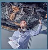
After the vehicle has been properly cleaned and prepared for treatment, carefully study the DINITROL spray diagram for the vehicle to be treated. This is the only way to avoid damage to the electrical system, airbags, and other sensitive parts.
