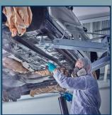
The cavities must first be treated using a penetrating, water-repelling DINITROL cavity protection product. Any excess material must be removed. The material needs 15–20 minutes to take effect and to penetrate the rust in the cavities and flanges.
