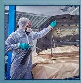
Once the cavity treatment is complete, the cavities of the boot door and bonnet must be sealed. Please ensure that the engine and boot are completely covered.
