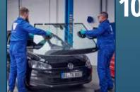
Insert the new windscreen within the adhesive's open time and use the tape to position it. Now install the associated components such as the trim, etc.
