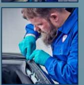
base. Please note: Do not treat the cut surface with open times of more than 12 hours, the trimmed bead must be cleaned with **DINITROL 582** and activated with **DINITROL 540**
