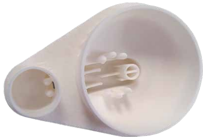
Fig. 5: Manifold with piercings for the foilwraps
