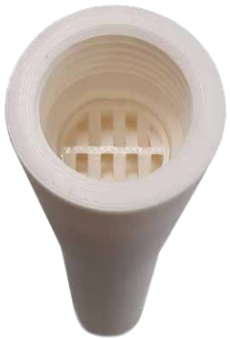
Fig. 6: Visible mixing elements in the mixer
