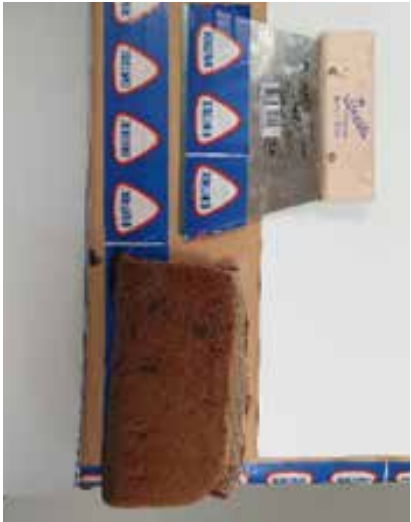
Fig. 5: Adhesive distributed with toothed trowel
