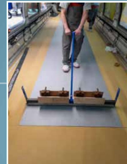
Fig. 10: Pressing the covering with the help of a roller
