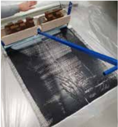
Fig. 4: Adhesive distribution with roller
