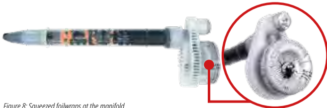
Figure 8: Squeezed foilwraps at the manifold
